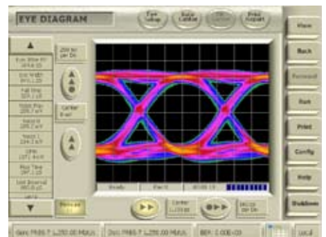
Fig. 2 Eye diagram of 50 m GI-PMMA-POF (OM-Giga) transmission at 1.25 Gbit/s
