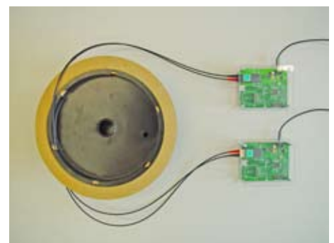
Fig. 3 Transmission of IEEE1394b over 50 m duplex GI-PMMA POF utilizing POF transceivers
