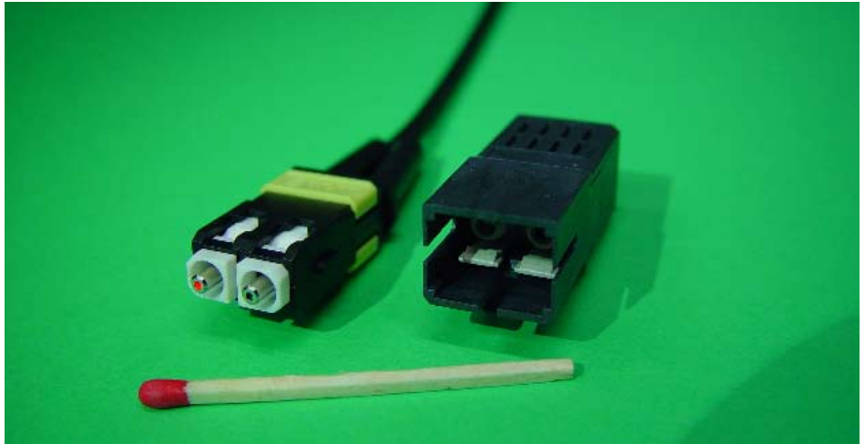
Fig.1 Gbit/s-Transceiver for duplex POF in SC-RJ-Package
