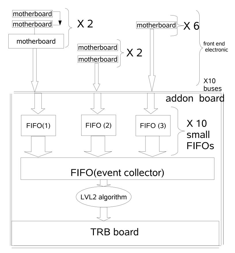
I take for example the DUBNA chamber: 14 short motherboards (8 TDC each) and 2 long moterboards (12 TDC each). At the end, I have 16 motherboards to read out or 136 TDCs
