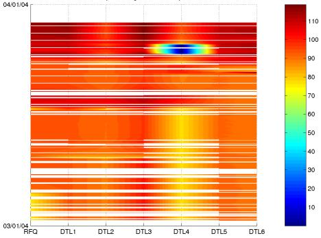
"Waterfall" Plot of SNS Transmitter Oil Tank Temperatures (Data averaged into 1000 bins)
