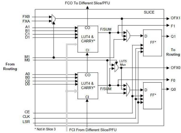
(c) Lattice FPGA slice diagram. [13]
