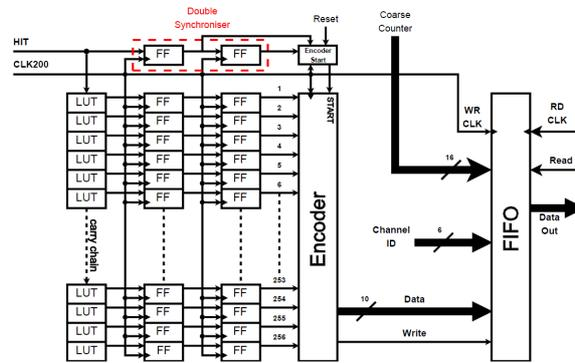
**Figure 2.** Diagram of a channel.
