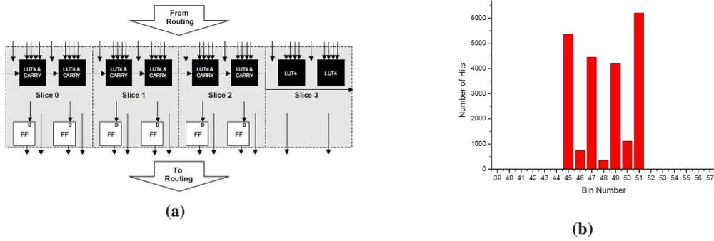
**Figure 5.** (a) Programmable Functional Unit of Lattice FPGA. [13] (b) Bin width pattern of a PFU.
