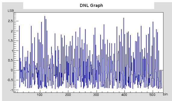
**Figure 8.** The differential non-linearity of the TDC.
