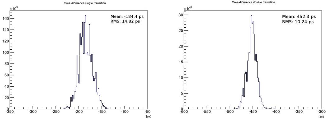
**Figure 7.** Time interval resolution of TDC with single and double transitions.
