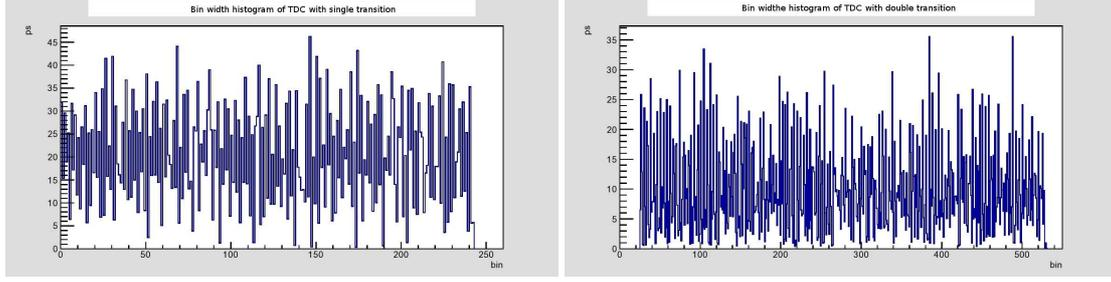
**Figure 6.** Bin width histogram for single and double transitions.
