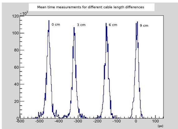
**Figure 9.** The shift of measured mean time with 3 cm cable length increase.
