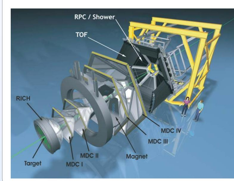
The HADES spectrometer is a versatile dielectron and hadron spectrometer located at the GSI Facility for heavy ion research in Darmstadt, Germany, and operational since 2002. The setup includes:
