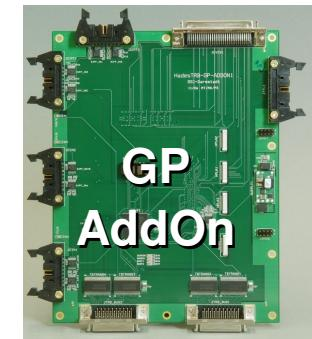
Trigger Box board, for HADES first level trigger decision, is under development. Currently General Purpose AddOn with TRB is used as a source of the trigger.
