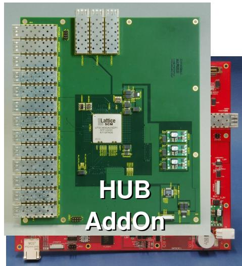
When several TRBs are working in one readout scheme, synchronization can be achieved by using one source of the trigger (Trigger Box). In such situation the optical HUB can distribute triggers.
