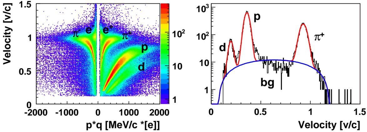
**Fig. 2.** Velocity vs. charge-times-momentum of charged particles as seen by the HADES detector from  $^{12}\text{C} + ^{12}\text{C}$  collisions at 2A GeV (left). Projection onto the velocity axis of positively charged particles with momenta  $350 \pm 5$  MeV/c and  $\theta = 60^\circ \pm 5^\circ$  (right). Fitted signal and background distributions are shown as lines.
