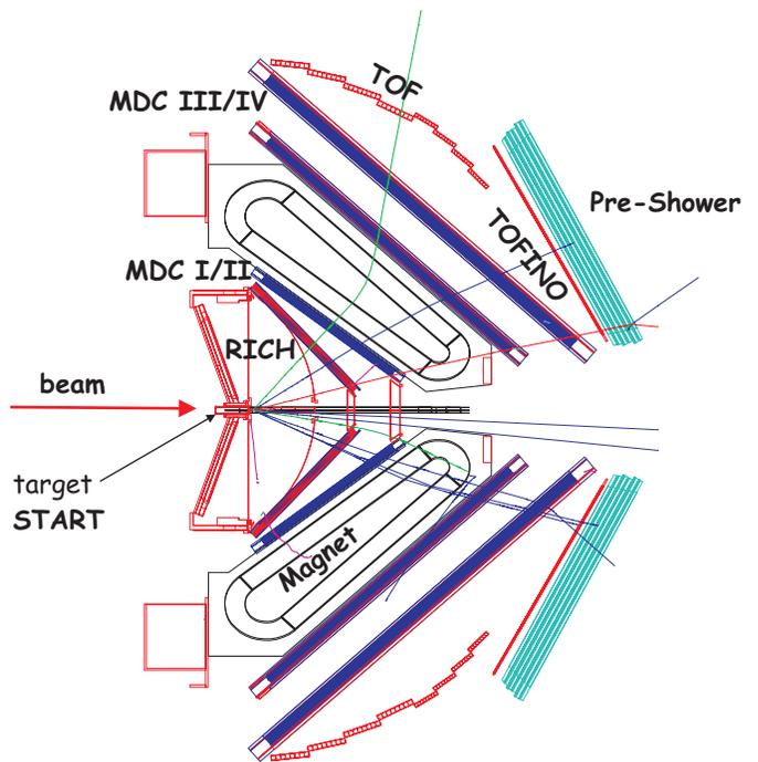
**Fig. 1.** Cut through two sectors of the HADES spectrometer, except for the magnet coils which are projected onto the cut plane to visualize the magnetic field. The average distance between the target and the outermost detectors is about 210 cm.
