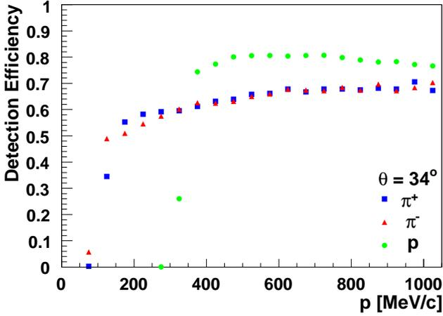
**Fig. 4.** The detection efficiency  $\varepsilon_t^{det}(p, \theta)$  vs. momentum for  $\pi^\pm$  and protons using the kickplane reconstruction in  $^{12}\text{C}+^{12}\text{C}$  collisions at 2A GeV.
